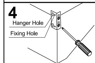
**4** Adjust hangers of both sides, hang machine onto screws and the fixing holes must be screwed on the wall.
